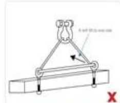
Figure 15. Do not tie the sling because eye back to another as it will not be safe.
