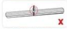
Figure 14. The hook will become side loading when it is not rigged correctly.
